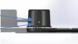
4. Keep the cabinet mounted 'operate' button pressed for 5 seconds.
